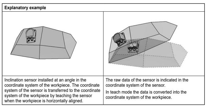
The example shows a rotation of 30° about the y axis of the coordinate system of the workpiece.
