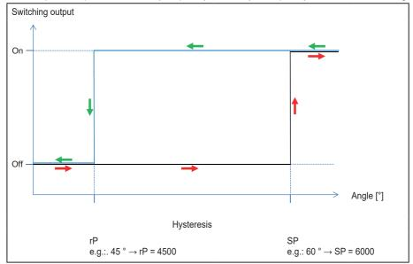
The respective parameter SP (set point) and rP (reset point) are used for setting.
