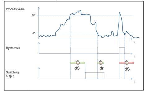
Switching and switch-off delay function
