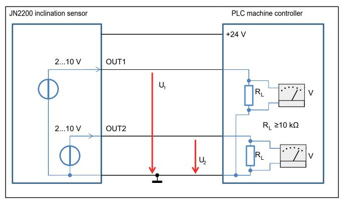
The measured values are implemented to the voltage intensity on the outputs as shown in the diagram below. Angle values smaller than the set start point are constantly mapped to the lowest value of 2 V. Angle values greater than the set end point are constantly mapped to the highest value of 10 V.
