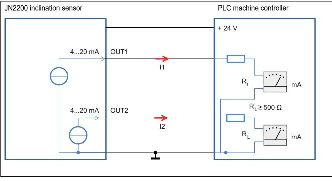
The measured values are implemented to the current intensity in the current loop as shown below. Angle values smaller than the set start point are constantly mapped to the lowest value of 4 mA. Angle values greater than the set end point are constantly mapped to the highest value of 20 mA.
