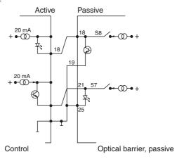
ON = input interface active, 20 mA current loop
