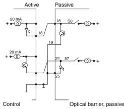
S7: ON = input interface active, 20 mA current loop
