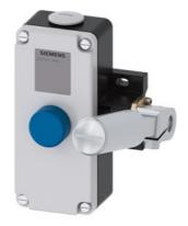
Conveyor belt unbalance tracker Metal enclosure, 2 x M25 x 1.5 2 NO+2 NC, with latching according to EN ISO 13850 Pushbutton release
