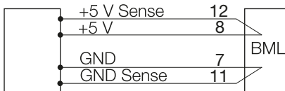
Fig. 4-5: Power supply with sense line
