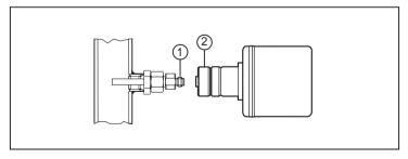
Attach the control monitor to the flow sensor (1).
