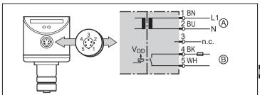
A: supply circuit B: output circuit
