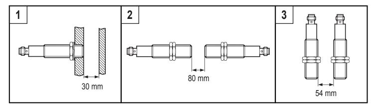
► Tighten the socket according to the manufacturer's indications. Observe the tightening torque for the ifm socket (e.g. EVxxxx: 0.6...1.5 Nm).
