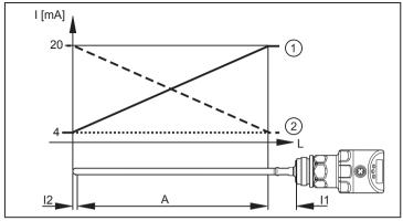
Curve of the analogue signal (measuring range scaled):
