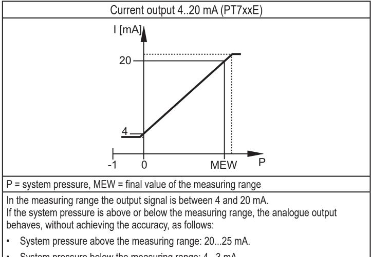
• System pressure below the measuring range: 4...3 mA.
