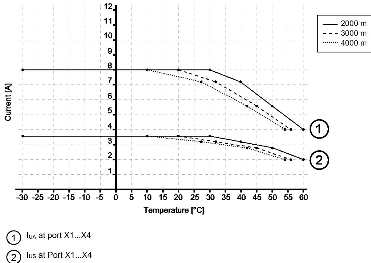
(1)  $I_{UA}$  at port X1...X4(2)  $I_{us}$  at Port X1...X4
