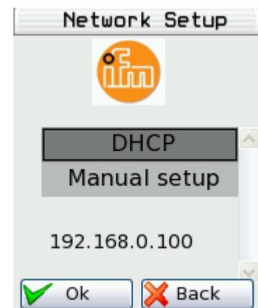
**Option 2: configure the IP parameters manually**
