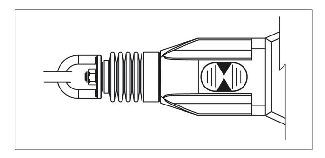
Rope tension indicator: Indicator shown with steel rope properly adjusted
