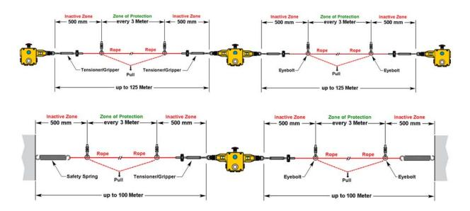
Installation of the components
