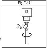
In case of high mechanical stress (strong vibration, moving viscous media) it may be necessary to secure the screw connection, e.g. by a screw retaining compound.
