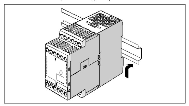
To avoid failures it is recommended to adhere to the operating temperature of the AS-i safety monitor for installation in control cabinets as specified in the technical data. In general it is recommended to adhere to a minimum distance of 10 mm between several safety monitors and to other control cabinet components.
