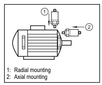
► Ensure safe vibration transmission and allow no elastic intermediate layers.
