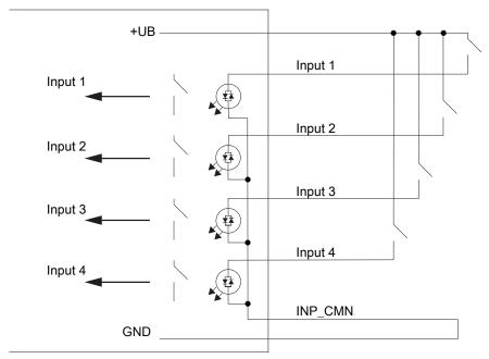
Fig. 4: Circuitry of the inputs not electrically isolated
