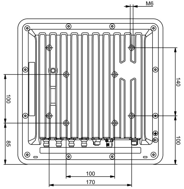
Fig. 1: Back with mounting holes
