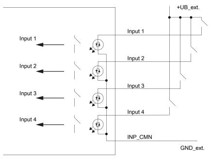
Fig. 3: Circuitry of the inputs electrically isolated
