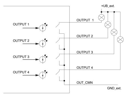
Fig. 5: Circuitry of the outputs electrically isolated
