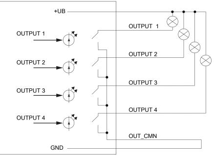
Fig. 6: Circuitry of the outputs not electrically isolated
