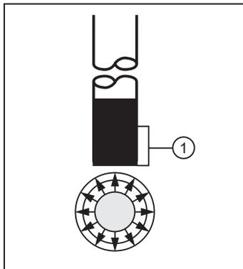
The device operates with radial detection characteristics. Therefore, media below the active zone (1) are not detected.
