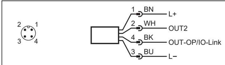
Fig. 1: Wiring diagram (colours to DIN EN 60947-5-2)
