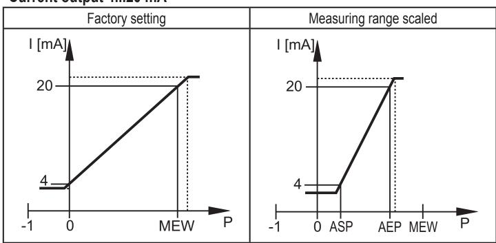
P = system pressure, MEW = final value of the measuring range In the set measuring range the output signal is between 4 and 20 mA. It is also indicated:
