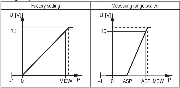
P = system pressure, MEW = final value of the measuring range In the set measuring range the output signal is between 0 and 10 V. It is also indicated:
