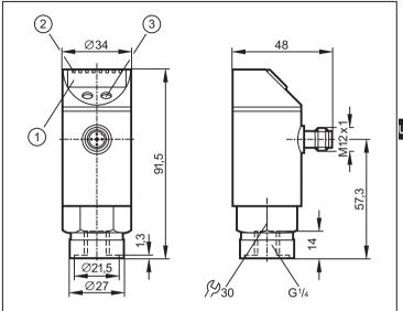
Dimensions are in millimeters
