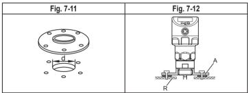
► Arrange for a bore hole in the tank lid. It must have a minimum diameter d to enable sufficient transfer of the measured signal to the probe (Fig. 7-11). The diameter (d) depends on the wall thickness of the tank lid:
