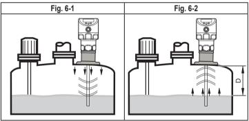
The unit operates on the principle of guided wave radar. It measures the level using electromagnetic pulses in the nanosecond range.
