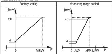
P = system pressure, MEW = final value of the measuring range In the set measuring range the output signal is between 4 and 20 mA. Also signalled:
