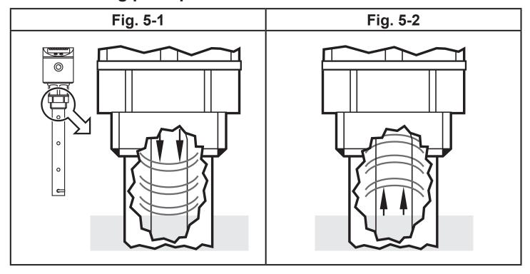
The unit operates on the principle of guided wave radar. It measures the level using electromagnetic pulses in the nanosecond range.
