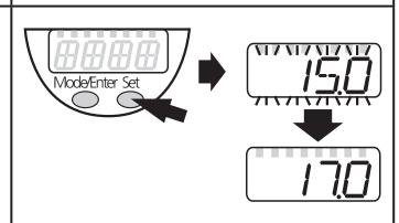
Numerical values are incremented continuously. For reducing the value: let the display move to the maximum setting value. Then the cycle starts again at the minimum setting value.
