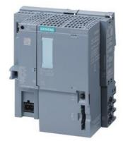
SIMATIC DP, CPU 1514SP-2 PN for ET 200SP, central processing unit with work memory 600 KB for program and 3.5 MB for data, 1st interface: PROFINET IRT with 2-port switch, 2nd interface: PROFINET RT, 6 ns bit performance, SIMATIC Memory Card required, BusAdapter required for 1st interface
