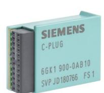
C-plug, removable data storage medium For simple device replacement in case of fault, for recording configuration or engineering and application data, can be used in the following SIMATIC NET products with C-plug slot: SCALANCE XC-200, XP-200, XM-400, XR-500, M-800, W-700, SC-600 and S615.
