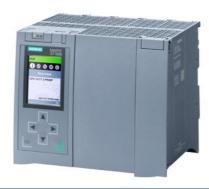
SIMATIC S7-1500T, CPU 1517T-3 PN/DP, Central processing unit with work memory 3 MB for program and 8 MB for data, 1st interface: PROFINET IRT with 2-port switch, 2nd interface, Ethernet, 3rd interface, PROFIBUS, 2 ns bit performance, SIMATIC Memory Card required
