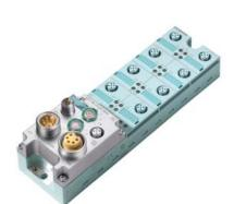
SIMATIC DP, basic module BM 142 ET 200ECO: 8 DO 24 V DC/2A; 8xM12, single assignment, Degree of protection IP65/67; Connection block 6ES7194-3AA00-0.A0 separately order
