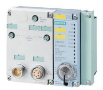
SIMATIC DP, CPU 1516PRO F-2 PN for ET 200pro, Central processing unit with work memory 1.5 MB for program and 5 MB for data, 1st interface: PROFINET IRT with 3-port switch, 2nd interface: PROFINET RT, 10 ns bit performance, degree of protection: IP65/67, SIMATIC Memory Card required, Connection module required
