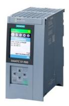
\*\*\* spare part \*\*\* SIMATIC S7-1500F, CPU 1516F-3 PN/DP, central processing unit with work memory 1.5 MB for program and 5 MB for data, 1st interface: PROFINET IRT with 2-port switch, 2nd interface: PROFINET RT, 3rd interface: PROFIBUS, 10 ns bit performance, SIMATIC Memory Card required
