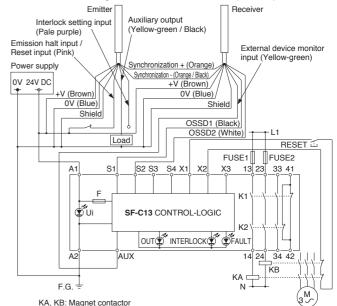
In case of connecting a type 2 PNP output type light curtain, connect the control output (OSSD) to S1, and also put a jumper between S2 and S3.
