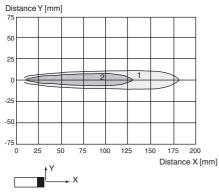
Curve 1: flat surface 10 mm x 10 mm Curve 2: round bar, Ø 8 mm
