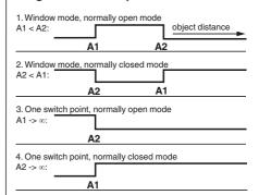
5. A1 ->  $\infty$ , A2 ->  $\infty$ : Object presence detection mode Object detected: Switch output closed No object detected: Switch output open
