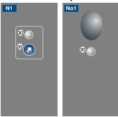
05 = Switching Distance Adjuster 30 = Switching Status/Contamination Warning
