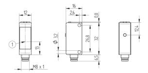
1= Optical axis M3 screw = 0.5 Nm Potentiometer = 40 Nmm Dimensions specified in mm (1 mm = 0.03937")
