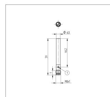
1 = Switching Status Indicator Sleeve 6,5 mm dia. = 8 Nm All dimensions in mm (1 mm = 0.03937 Inch)
