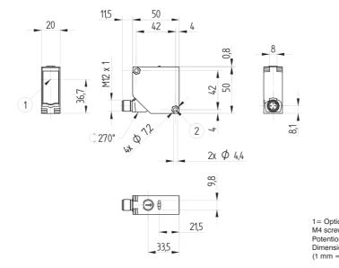
1= Optical axis M4 screw = 0.5 Nm Potentiometer = 40 Nmm Dimensions specified in mm (1 mm = 0.03937")
