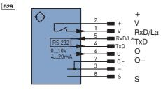
Supply Voltage + Contamination/Error output (NO) RS-232 Receive Line/Emitted light disengageable RS-232 Transmit Line Analogue output Ground for the analogue output Supply Voltage 0 V Shielding
