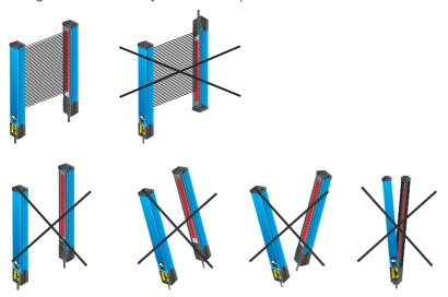
Correct alignment is indicated by the bar graph at the display. When all beams are shown as uninterrupted, the Light Barrier is correctly aligned.
