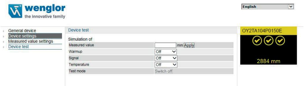
The screenshot displays the 'Device test' configuration page. On the left, a sidebar menu lists 'General device', 'Device settings', 'Measured value settings', and 'Device test'. The 'Device test' section is active, showing a table of parameters:
