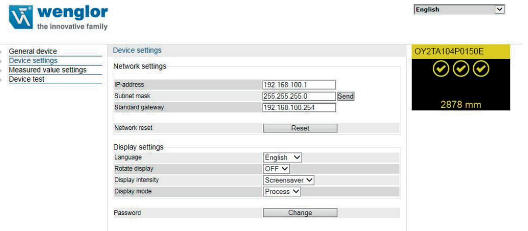
The screenshot shows the 'Device settings' configuration page. On the left is a navigation menu with options: General device, Device settings, Measured value settings, and Device test. The main content area is titled 'Device settings' and is divided into two sections: 'Network settings' and 'Display settings'.
