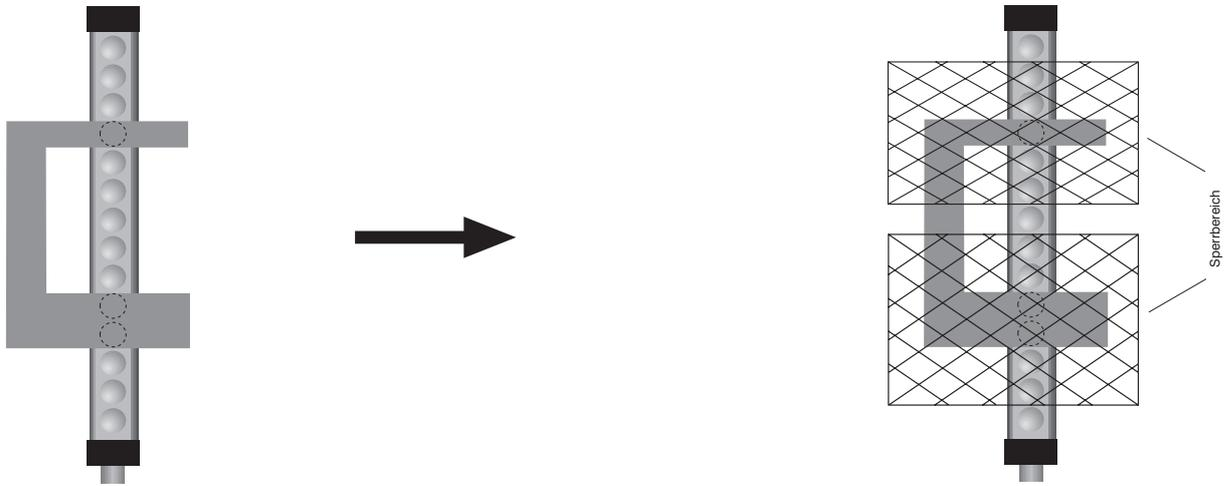
If penetration into the exclusion zone is not possible, light curtain resolution remains unchanged.
