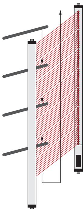
Each light beam between the emitter and the receiver must be inspected by obstructing each beam with the test rod. The test rod must be moved slowly through the safety field in accordance with the adjacent diagram.
