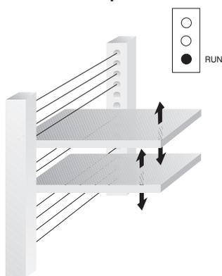
Up to 3 objects can pass through the safety field without causing the safety output to switch. The beams which are obstructed by the objects are adapted to the respective size of the object, and are muted accordingly.
