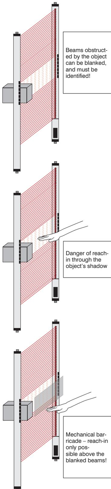
A fixed object is always located at the same position within the safety field. The beams which are obstructed by this object can be blanked.
