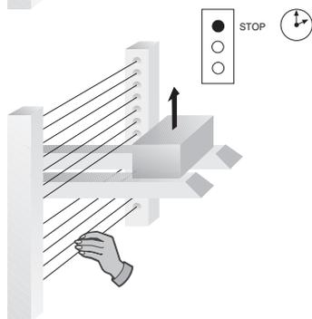
The safety output is switched when additional beams above and beyond the blanked beams have been interrupted, for example if someone reaches into the safety field.
