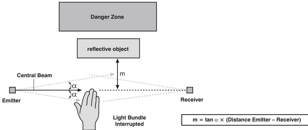
$\alpha$  = aperture angle of emitter and receiver optics
