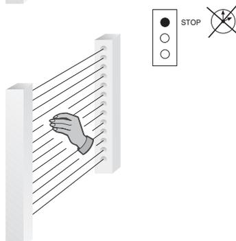
The safety output is switched if the safety field is penetrated at the middle.
