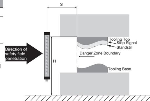
**A minimum clearance of S = 100 mm must be maintained (resolution ≤ 14 mm)**
