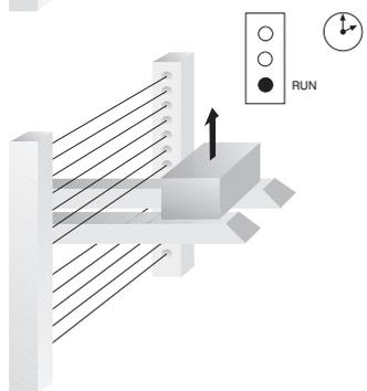
**The order in which safety field beams are obstructed must always start at the top or the bottom.**
