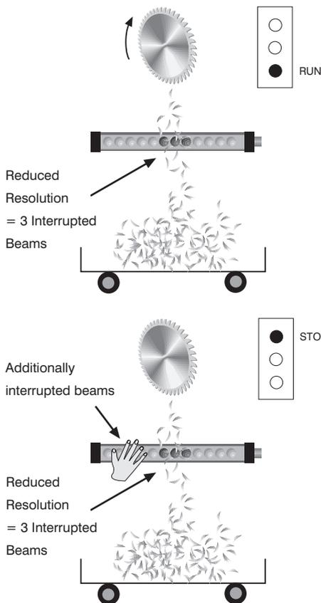
A certain number of adjacent beams can be interrupted with reduced resolution without causing the safety output to switch (see table). Light curtain resolution is thus changed.
