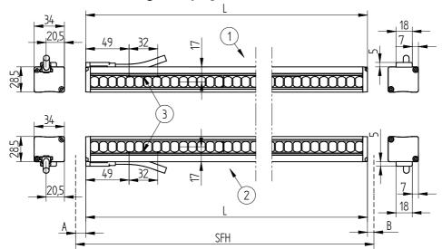
1 = emitter, 2 = receiver, 3 = control panel, SFH = safety field height
