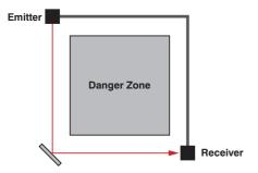
The range of possible applications can be significantly expanded through the use of a Deflection Mirror. Deflection Mirrors are available in two different variants:
