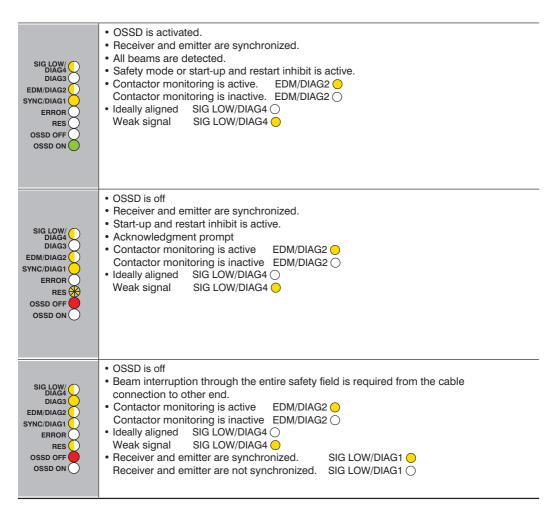
When the maximum range of the sensors is exploited, "SIG LOW/DIAG4" may appear at the display even if they are ideally aligned.
