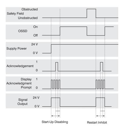
$t_{\scriptscriptstyle 1}$  - Acknowledgement duration: 0.1 to 4 s  $t_{\scriptscriptstyle 2}$  - On-time: 30 to 120 ms
