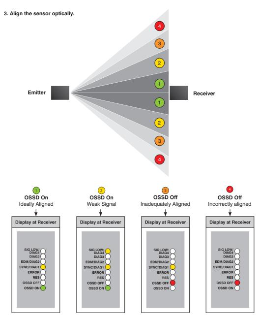
When the maximum range of the sensors is exploited, "SIG LOW/DIAG4" may appear at the display even if they are ideally aligned.
