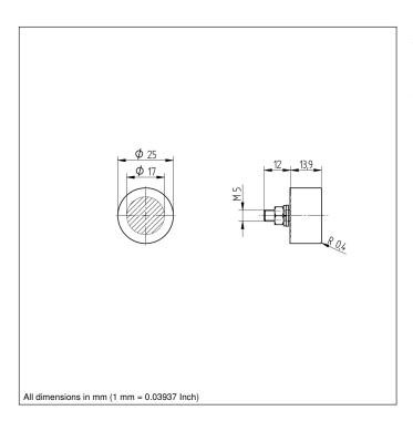
InoxSens is the hygiene series from wenglor. Together with other components, wenglor's InoxSens reflectors in stainless steel protection housing are part of this complete system which is seamlessly integrated into the machine. The reflectors are furnished with IP68 and IP69K protection and are attached using either InoxLock or fixing screws.
