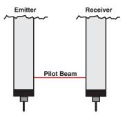
The purpose of adjustment is to accurately set the light curtain receiver to the required range. Adjustment must be performed after mechanical installation of the light curtain. After the light curtain has been adjusted, it immediately switches to the respectively selected operating state as soon as supply power is applied.
