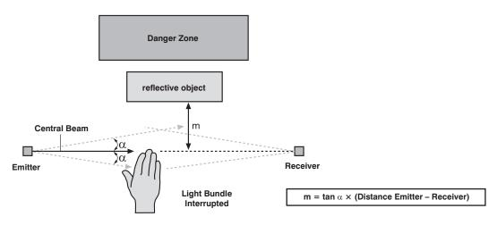
$\alpha$  = aperture angle of emitter and receiver optics  $\alpha$  = ±2,5°
