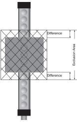
If penetration into the exclusion area is possible, resulting resolution (max. number of floating beams) amounts to 6 beams in the example (resulting resolution = 56 mm, see "Resulting Resolution" table).
