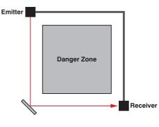
Possible applications can be significantly expanded through the use of a path-folding mirror. These path-folding mirrors are available in two different variants:
