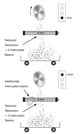
A certain number of adjacent beams can be interrupted with reduced resolution without causing the safety output to switch (see table). Light curtain resolution is thus changed.
