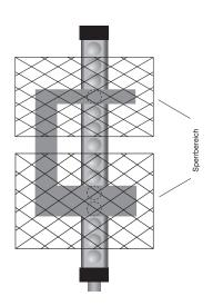
If penetration into the exclusion zone is not possible, light curtain resolution remains unchanged. The maximum number of floating beams is otherwise used to determine resolution.
