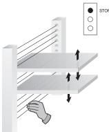
The safety output is not switched until additional beams above and beyond the blanked beams have been interrupted, for example if someone reaches into the safety field
