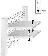
Up to 3 objects can pass through the safety field without causing the safety output to switch. The beams which are obstructed by the objects are adapted to the respective size of the object, and are muted accordingly.
