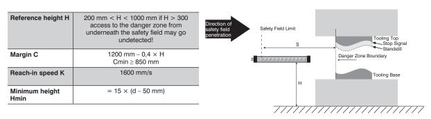
Required safety light curtain resolution for any given height must thus be calculated as follows.
