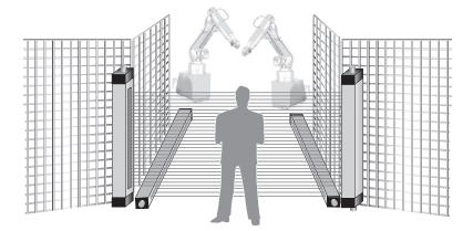
Example: securing off an area plus side-stepping protection
