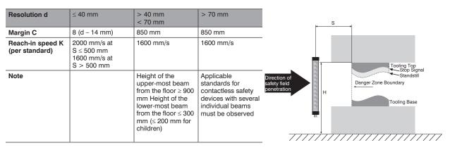
A minimum clearance of S = 100 mm must be maintained (resolution  $\leq$  14 mm) A minimum clearance of S = 150 mm must be maintained (resolution  $\leq$  30 mm)
