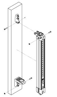
First secure the mounting clamp to the Light Curtain with the screws. The screws should remain accessible after mounting. In this way, the Light Curtain can be adjusted at a later point in time.
