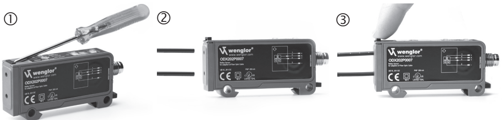
fig. 3 Connecting the plastic fibre-optic cable
