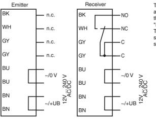
The relay-functions "NC" and "NO" bear on the switching mode "Dark-ON". This complies to the default setting of the light/dark switch (factory setting).
