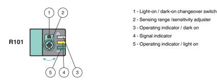
To unlock the adjustment functions turn the sensing range adjuster for more than 180 degrees.
