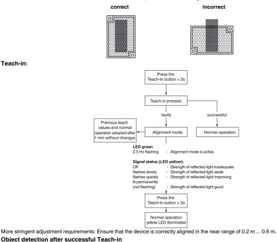
The target should be large enough so that the reflector is always completely covered in one dimension! optimal
