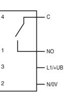
The relay-functions "NC" and "NO" bear on the switching mode "Dark-ON". This complies to the default setting of the light/dark switch (factory setting).
