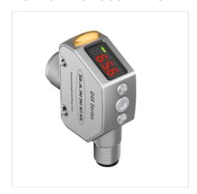
Q4X Series: Laser Adjustable Field Range: 100 mm; Input 10-30 V dc Outputs: Bipolar: 1 NPN; 1 PNP
