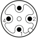
Fig. 4-1: Pin assignment of S4 connector (view from above on connector of BIP)
